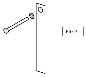
3) FEED A WASHER ONTO THE SCREW OR BOLT YOU SUPPLY, THEN FEED ONE COMPLETE STRAP ASSEMBLY ONTO THAT SAME SCREW OR BOLT. MAKE SURE THAT THE SHOW SIDE OF THE BUCKLE FACES YOU. (See fig.3)
